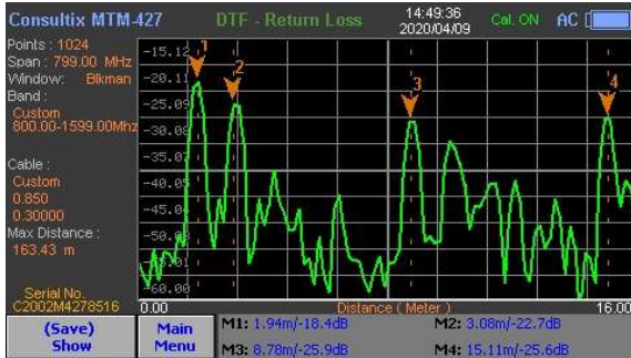
Figure 10.a. DTF with wrong cable settings
