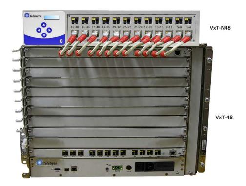
The VxT-N48 (top unit) is shown connected via 12 short Category-7 jumper cables to the VxT-48 xTalk Emulator for VDSL2 Vectoring Testing (bottom unit). Another VxT-N48 may be placed below the Emulator (in a rack) for injection on the other side of the loop. This product may also be used with Telebyte's local loop simulators.
