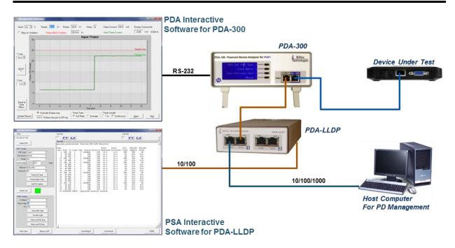
The **PDA-LLDP** is used to assess PoE LLDP protocol from a Powered Device (PD). It is readily used in tandem with a **PDA-300** that provides power to the PD and monitors (or charts) it's real-time power loading, including load state changes that might be resultant from PoE LLDP negotiation and power adjusts. For further information regarding the PDA-300 from Sifos, see the **PDA-300 Product Overview** available at www.sifos.com.
