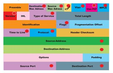
The red dot marked fields can be used as a match for a packet, stand-alone, combined or with wild cards. For IP Src and IP Dst super nets are supported.
