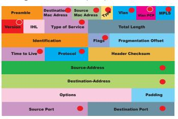
The red dot marked fields can be used as match for a packet, stand-alone, combined or with wild cards. For IP Src and IP Dst super nets are supported.
