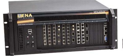
Available in both a 1U and 4U form factor, the high-density Xena chassis can be equipped with a wide variety of test modules.
