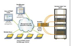
complete test platform for wire speed test load generation and analysis. Key features include wire-speed traffic generation and analysis, a GUI framework, an open TCP/IP scripting protocol, and integration with a broad range of functional and conformance test suites.
