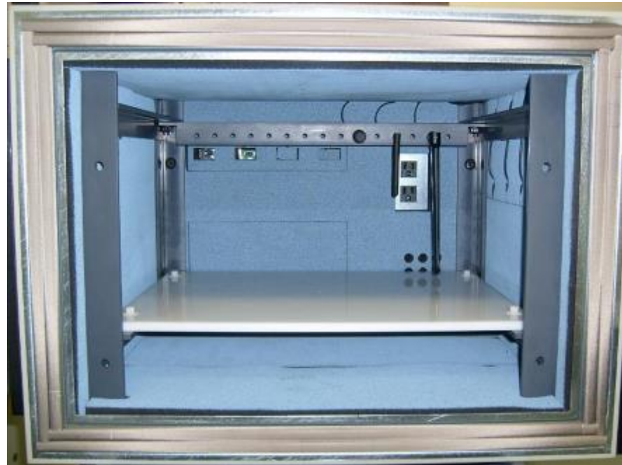
Dual gasketing and right angle door seals
