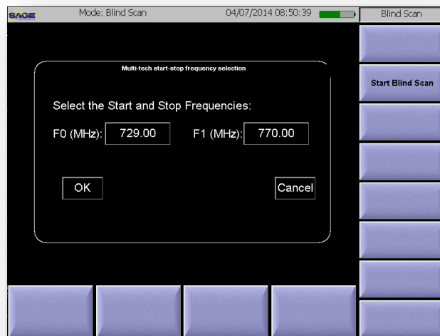
Figure 5 Shows Blind Scan User Selectable Frequency Scan Range
