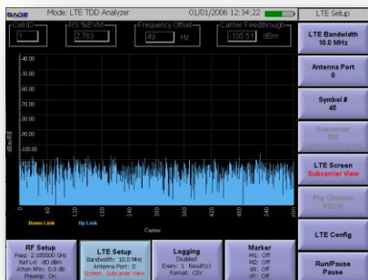
Figure 7 LTE-TDD SubCarrier View. [No Activity, SP 45]
