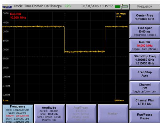
Figure 15 Shows Zero-Span of 10 MHz LTE-TDD
