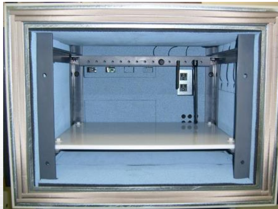
Dual gasketing and right angle door seals
