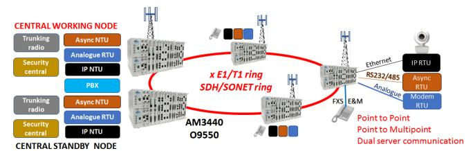
Many installations in Oil and Gaz or Chemical complex are managing the process control and SCADA over Ethernet RTU. But as the site was installed more than 10/20 years ago several applications are always based on analog RTU, or with integrated modem to provide the timing information or low rate asynchronous or synchronous communication. The Loop DACS care for all applications and provide the absolute QoS for application based also on IP transport.
