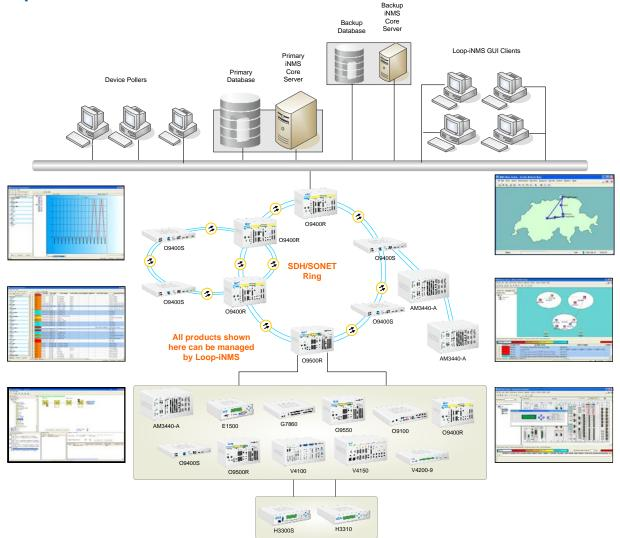
The Loop-iNMS basic components are Device Poller, iNMS core and iNMS GUI Clients as shown in the top part of the diagram. The Loop-iNMS is capable of managing all the devices from Loop.
