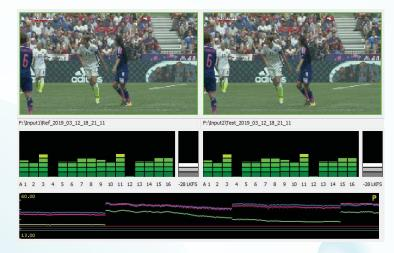
The RTM 4K presents a significant technological breakthrough by applying a fully uncompressed 4K video source with embedded audio and performing a real-time video PSNR or DMOS via comparison to a 4K encoded/decoded signal input along with audio quality, lip sync and audio program loudness measurements at the same time.
