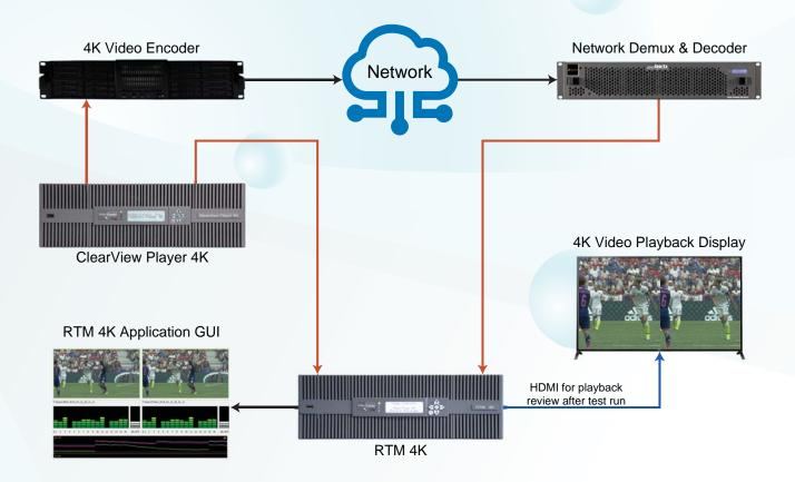
Real-Time Quality Testing for Network 4K Encoder or Transcoder
