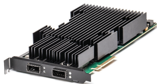
The seven speed Thor-400G-7S-1P test module can test 400GE / 200GE / 100GE / 50GE / 40GE / 25GE / 10GE
