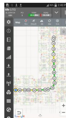
Figure 4, Modulated Walk Test Done by WTX-610 iLLuminator @ EARFCN=1301 & PCI = 3
