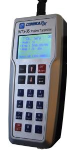
Consultix's award-winning CellWizard™ Test Transmitters are setting the standard for next generation transmitters for indoor and outdoor applications. The wideband operation frequency allows a single device to be used for all bands and technologies from 60MHz and up to 3 GHz, eliminating the need to purchase and carry multiple transmitters to the site.
