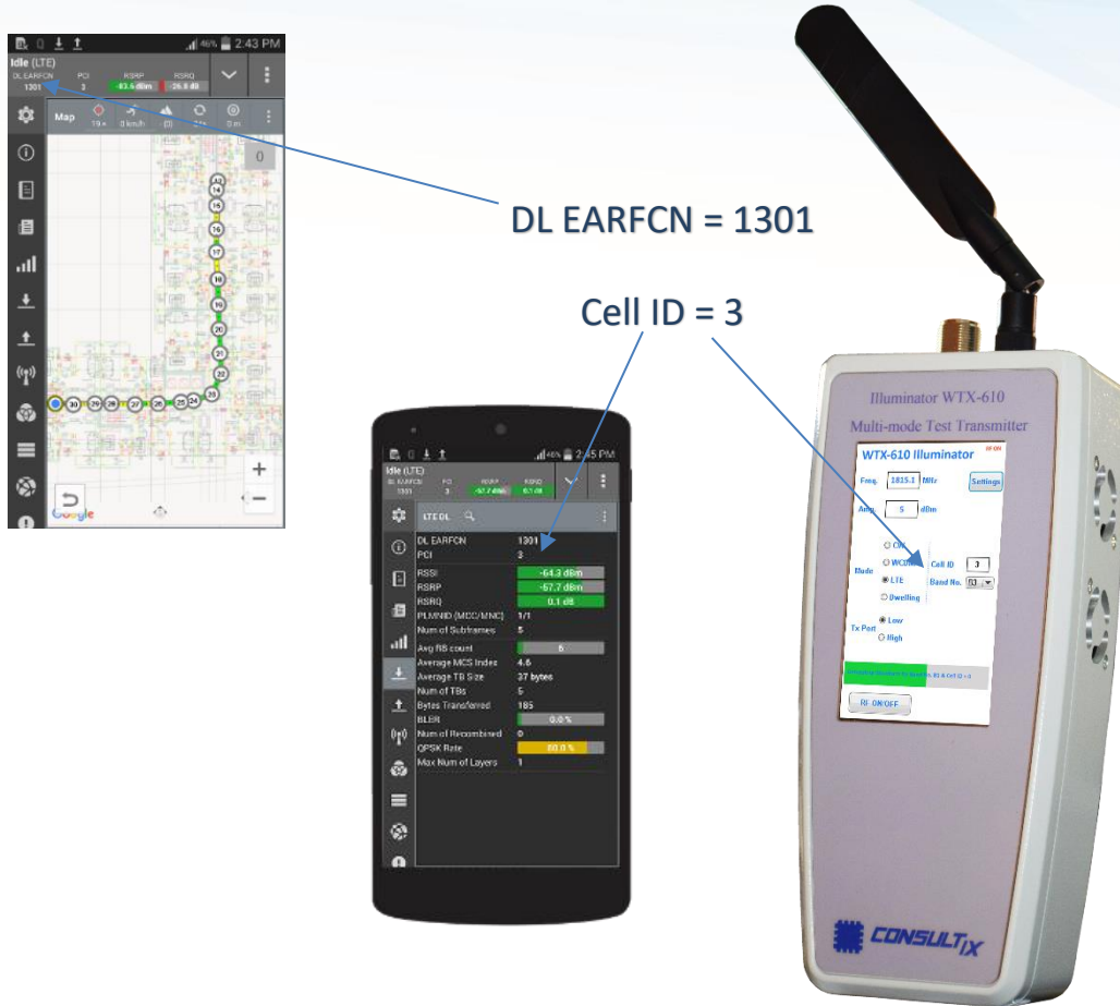
Figure 5: A complete Modulated Walk Test using ILLUMINATOR and test phone
