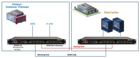
The MSM10G-R module is equipped with 4 Small form factor Pluggable slots for optical SFP or SFP+ modules. Dual Channel mode with dual sided protection
