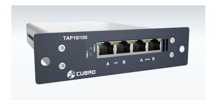
The Cubro fast ethernet 10/100 Copper TAP provides passive monitoring access to a single full-duplex network. The copper network TAP provides the highest performing and most cost-effective access to devices for passively monitoring your network. The TAP has 100 % throughput, very low delay and fully transparent, even for layer 1 and layer 2 faults.
