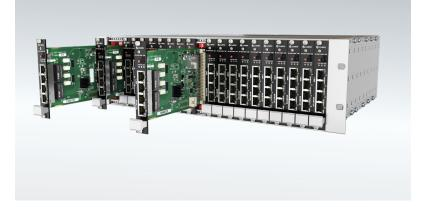
Cubro FlexTAP T-100 provides a copy of the packets (which are running through the data link) at the monitor outputs. The FlexTAP monitors the data link traffic anytime without any interruptions (to the data link). Further, a FlexTAP can be used to analyse "real traffic" in data links under real life (e.g. full load) conditions at any time it is desired or necessary.
