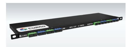
Cubro's MTP/MPO TAPs are passive fibre breakout TAPs that make an identical copy of your network's data, allowing your monitoring tools to see every bit, byte and packet. The small form of the TAPs allows to combine up to three different Slimline (different splitting ratio, or different connectors) TAPs in one RU.
