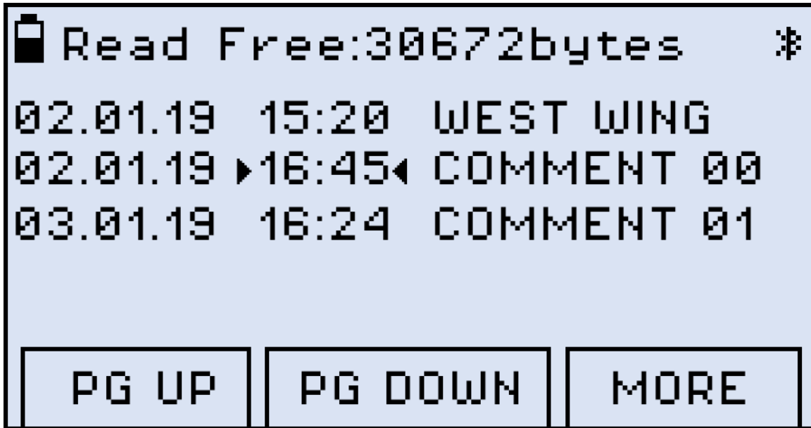
Viewing Measurement Results (Read mode)
