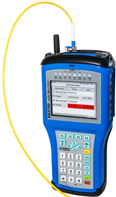
Image shows KE3700 with optical fibre module
