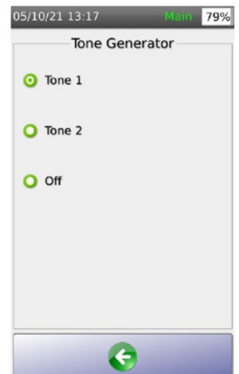
Figure 6 - Tone Generation option offers varying Tone options to be received by the filtering Tone Probe.
