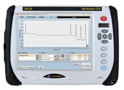
The LOR-220 from Luciol Instruments is a fully portable high resolution OTDR. It is similar in shape and feel to a standard OTDR, but achieves unprecedented resolution. The LOR-220 distinguishes events with 10 cm separation and has a 40 cm attenuation deadzone. Its unique dynamic range for short pulse lengths (over 14 dB for 1 ns pulses) enables to see through optical splitters, even over very short distances.
