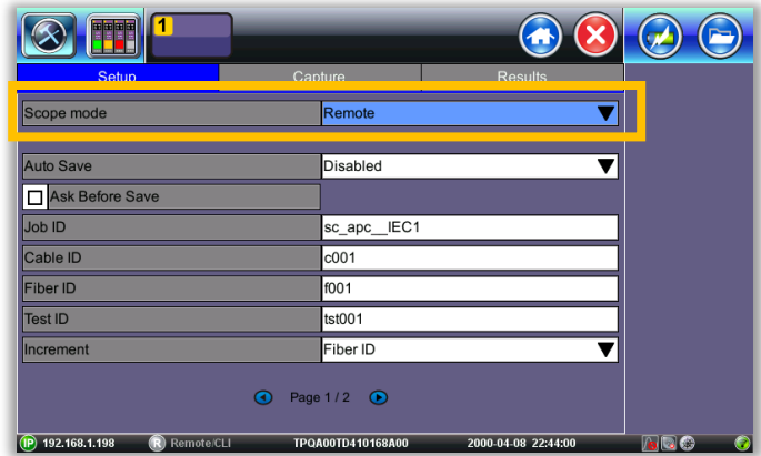
Figure 6: V150 Platform WiFi setup (Fiber Scope Setup)
