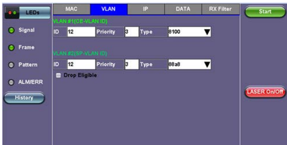
BERT Setup - VLAN Tag configuration (Layer 2 & 3)
