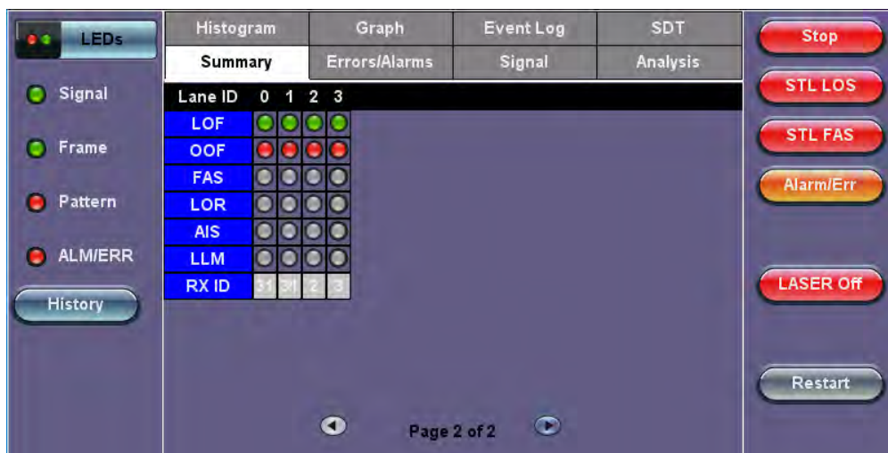
Summary displaying alarms/errors per lane
