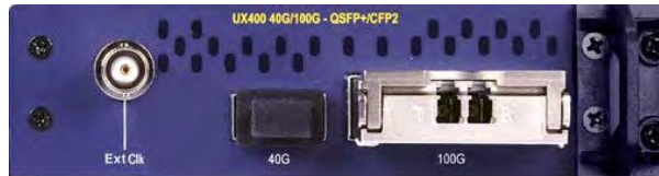
UX400-100G QSFP+ and CFP2 connector panel
