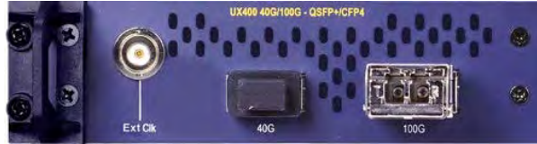
UX400-100G QSFP+ and CFP4 connector panel
