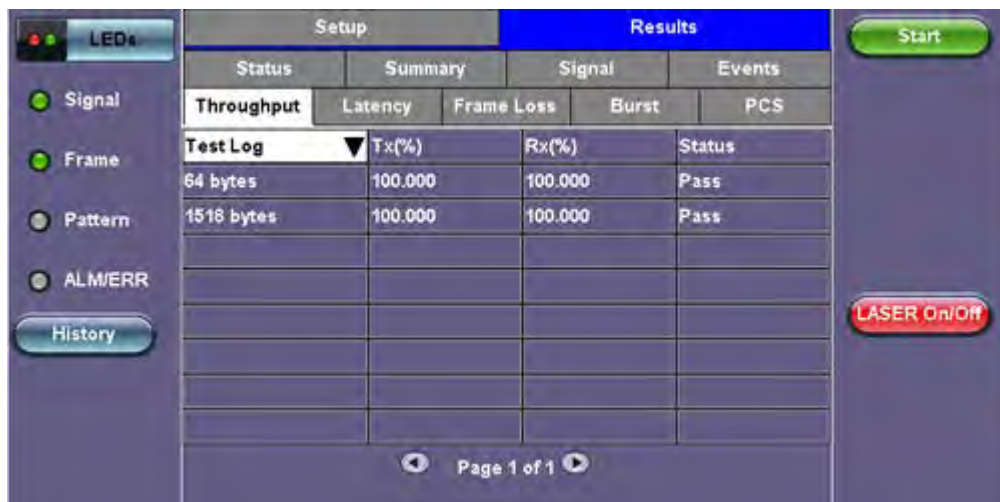
RFC2544 Results Throughput Test Log
