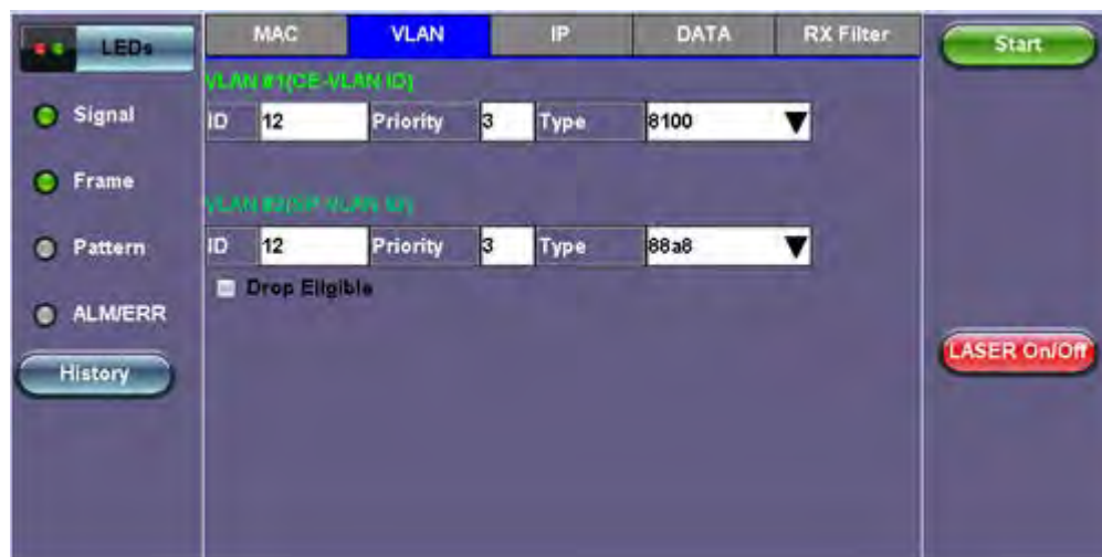
BERT Setup - VLAN Tag configuration (Layer 2 & 3)
