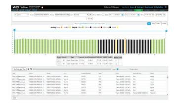
Measured data is stored in the VeSion sytem database for an extended period of up to 200 days, depending on the capacity of hard disk which can be configured by the system administrator. Archived data can be recalled and correlated with current alarm condition in live play back mode.
