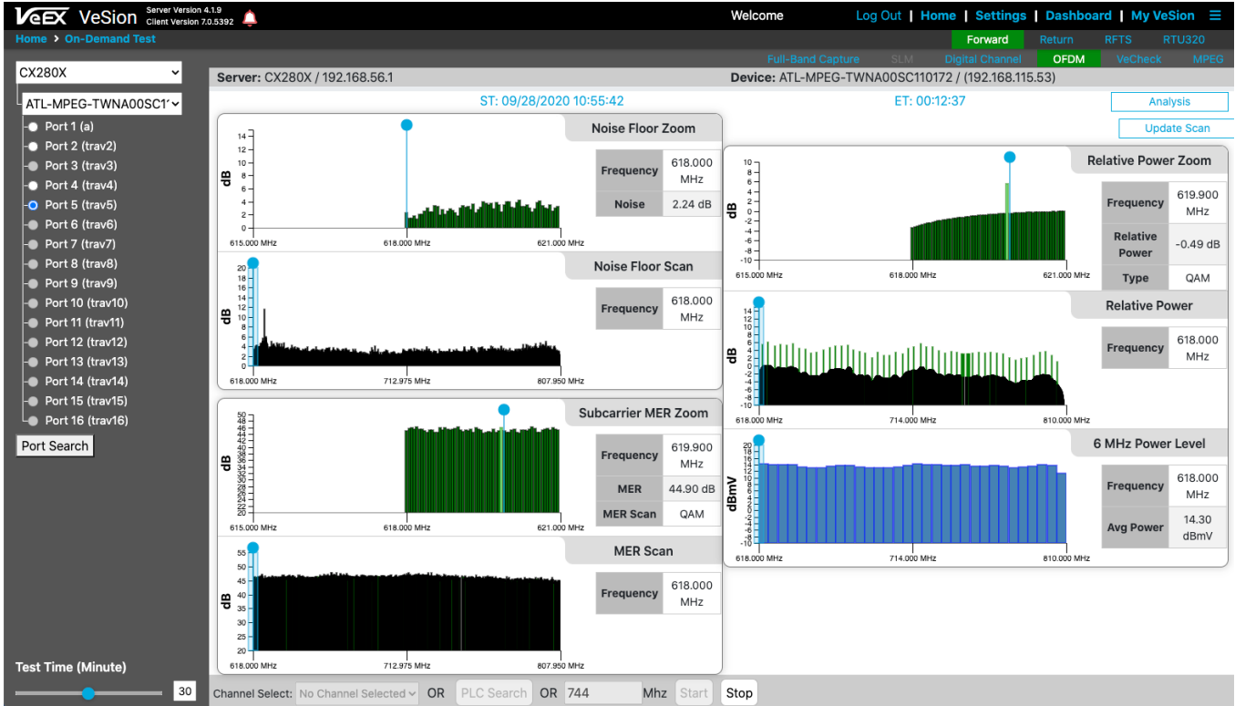
Subcarrier Scan: OFDM On-Demand Test screen
