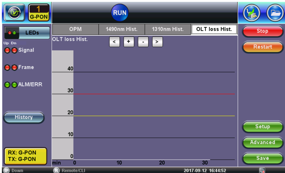
OLT Loss Histogram showing Downstream and Upstream signals
