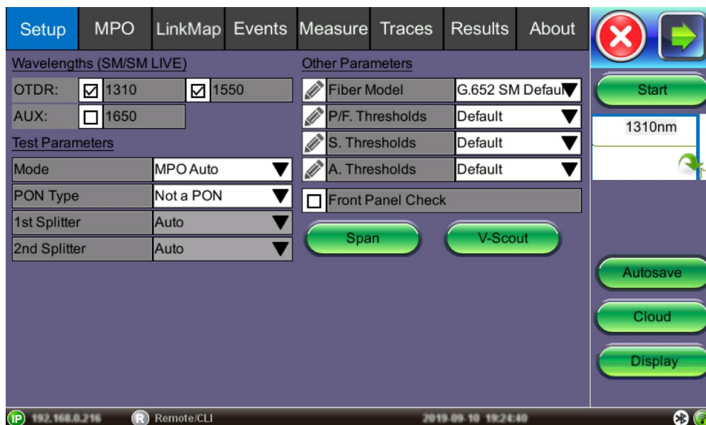
OTDR Screen (with MPO switch connected)
