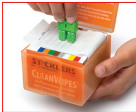
Clean the connector end-face by rubbing it onto a lint-free wipe dampened with isopropyl alcohol
