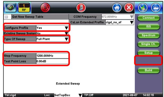
Figure 3: CX380C Full Plant Sweep Profile Setup
