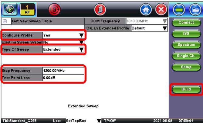
Figure 2: CX380C Extended Sweep Profile Setup
