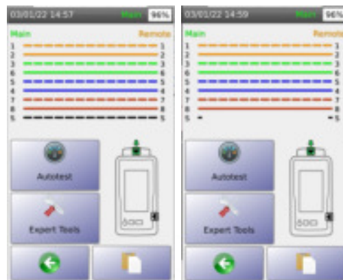
Fig 2 - Cable with good shielding and broken shield (DC shield discontinuity)
