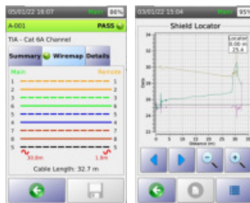
Fig 3 - Cable with AC shielding discontinuity and its time domain locator plot
