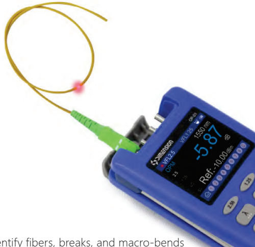
To identify fibers, breaks, and macro-bends
