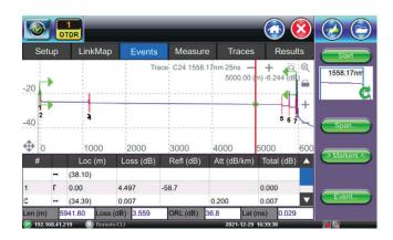
The unit employs specialized software algorithms developed from years of experience to measure fiber attenuation including anomalies such as connectors, splices, and macro-bends.
