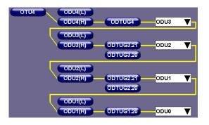
OTU4 Single-step mapping/multiplex structures
