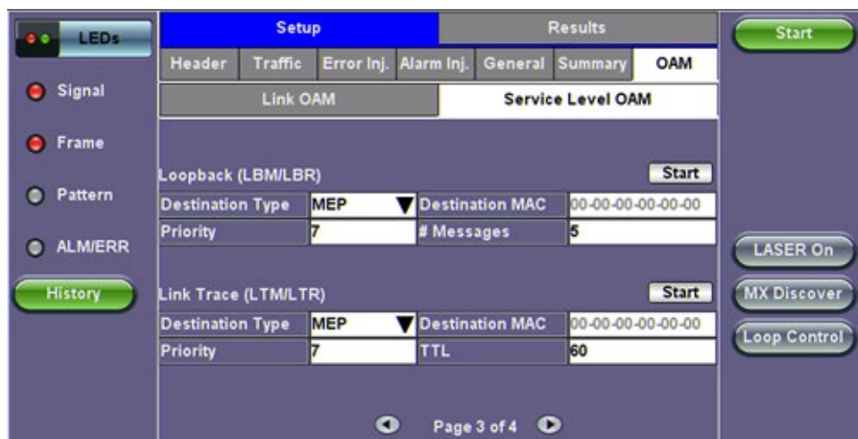
Pressing Start next to Loopback (LBM/LBR) initiates testing for that OAM service
