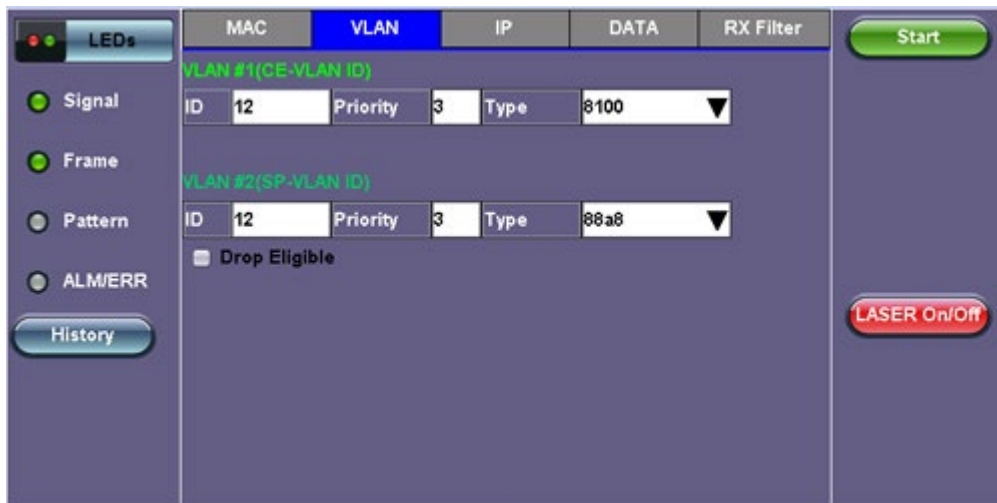
BERT Setup - VLAN Tag configuration (Layer 2 & 3)
