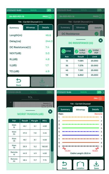
TestPro supports testing and certification for network deployments up to 40 Gigabit Ethernet for Cat3 through Cat8.2 or Class I/II cabling system. The electrically centered test plug assures the Level 2G/VI accuracy required to support field testing to Cat 8 / Class I/II, and actually exceeds the 2000 MHz requirement, to offer a 3000 MHz platform. The 3000 MHz frequency range provides investment protection as standards evolve, the test platform is ready.
