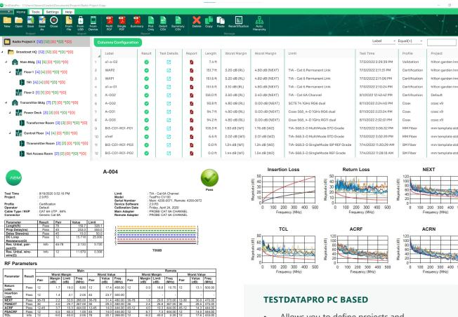
TestDataPro supports both PC and cloud-based options, and is included with all models of TestPro. Printed test reports for copper and fiber optic include a listed of compliant network support based on the performance of the cable tested.
