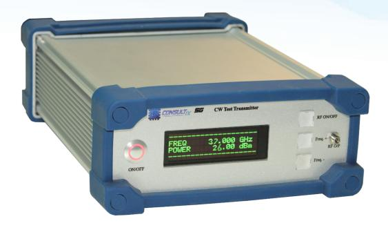
5G-Duo test transmitter is a portable 26 dBm signal generator that brings simplicity and affordability to mmWave test scenarios required for 5G propagation studies and model calibration.
