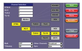
PDH/DSn client can be multiplexed and mapped into SDH/ SONET, which in turn can be mapped and multiplexed into OTN using synchronous or asynchronous modes. In synchronous mode the Optical Payload Unit (OPU) clock is derived from the mapped client signal while in asynchronous the OPU clock is independent.
