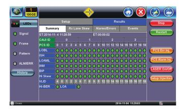
Example of 100GE Layer 2 100% throughput test result display
