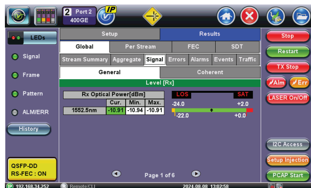
New TX Power Level in the Signal tab
